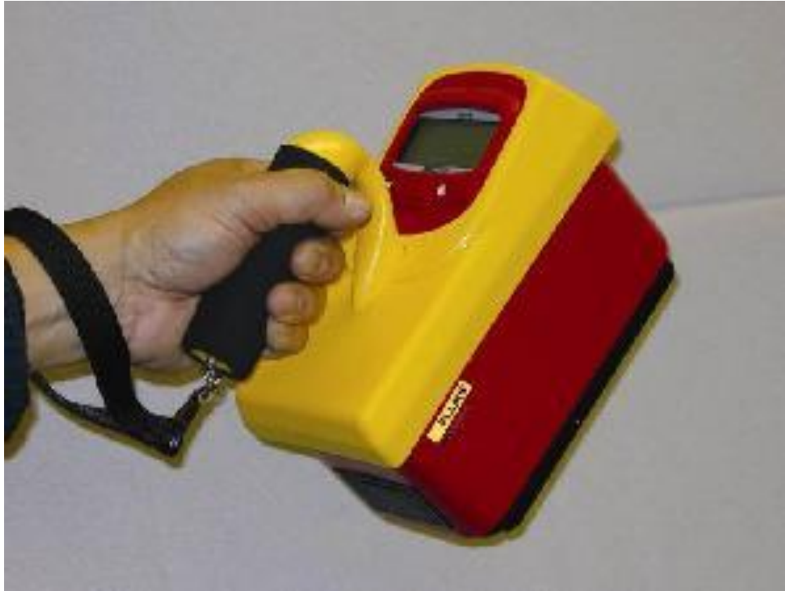
Ionization Chamber Model 451B manufactured by Fluke Biomedical
