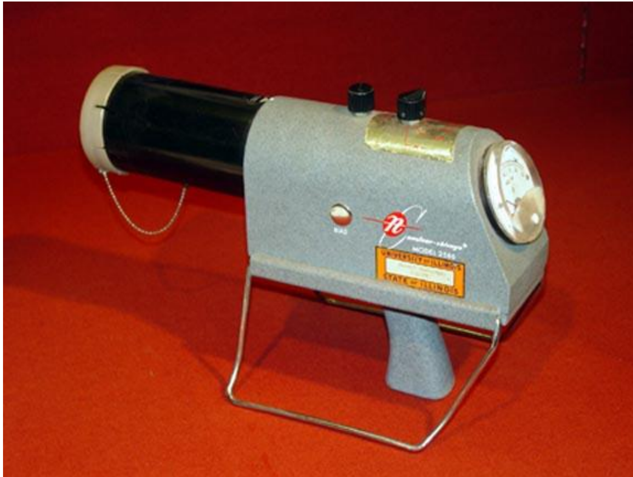
Ionization Chamber "Cutie Pie" manufactured by Nuclear Chicago
